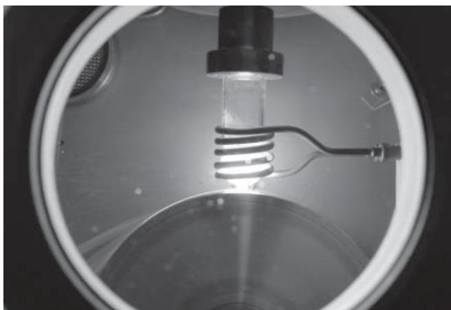
**The researchers rely on the melt spinning process for the recycling of permanent magnets. For this, the material is melted in a crucible using an induction coil and subsequently poured onto a copper wheel. (© Fraunhofer Project Group IWKS) | Picture in color and printing quality: [www.fraunhofer.de/press](http://www.fraunhofer.de/press)**
