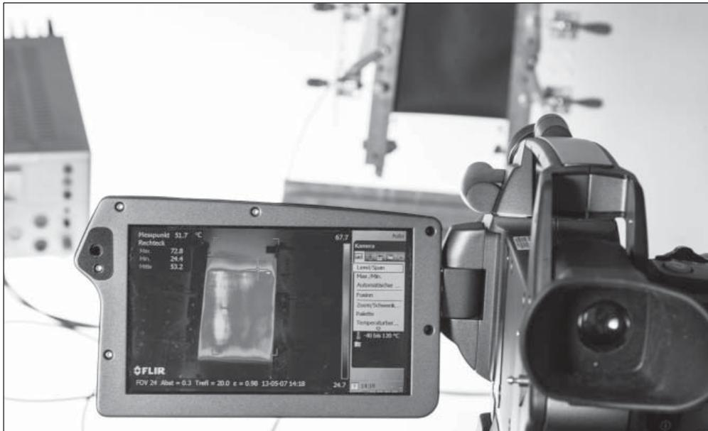
In order to analyze the heating effect of the films for cars, the researchers connected them to a power source and monitored them using a thermo camera. (© Fraunhofer IPA) | Picture in color and printing quality: [www.fraunhofer.de/press](http://www.fraunhofer.de/press)
