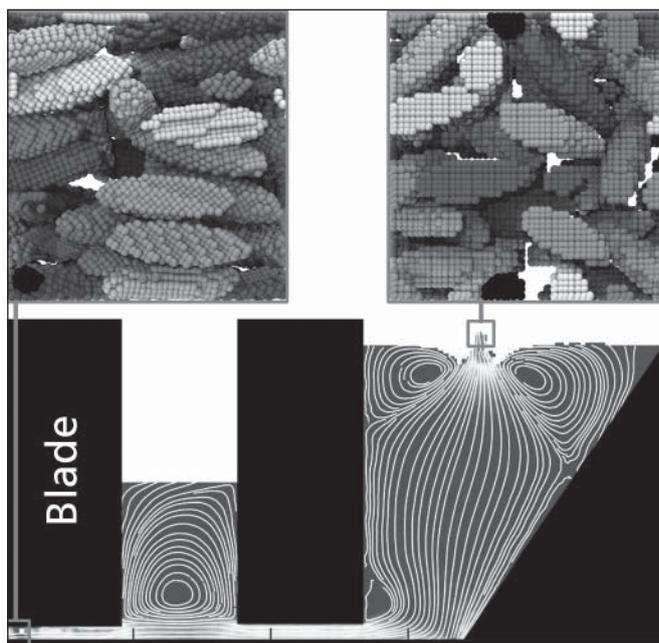
**Bottom – macroscopic simulation: flow lines during the casting process. The ceramic slurry enters the system on the right and exits the casting chamber on the left as a tape. Top – microscopic simulation: alignment of the ceramic particles at two points in the process. (© Fraunhofer IWM) | Picture in color and printing quality: [www.fraunhofer.de/press](http://www.fraunhofer.de/press)**
