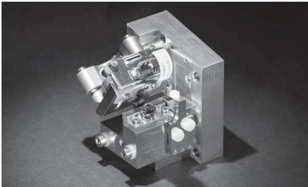
Scientists will soon be tracking the course of chemical reactions in real time. A quantum cascade laser, which records 1,000 spectra/second, makes it all possible. (© Fraunhofer IAF) | Picture in color and printing quality: [www.fraunhofer.de/press](http://www.fraunhofer.de/press)
