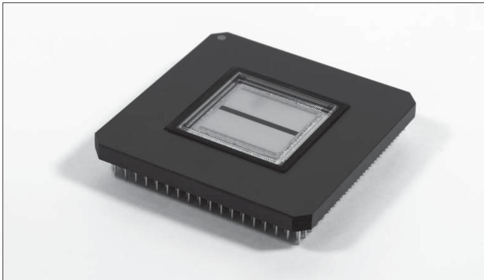
**This 60-line sensor is twice as fast as previous systems. (© Fraunhofer IMS) | Picture in color and printing quality: [www.fraunhofer.de/press](http://www.fraunhofer.de/press)**
