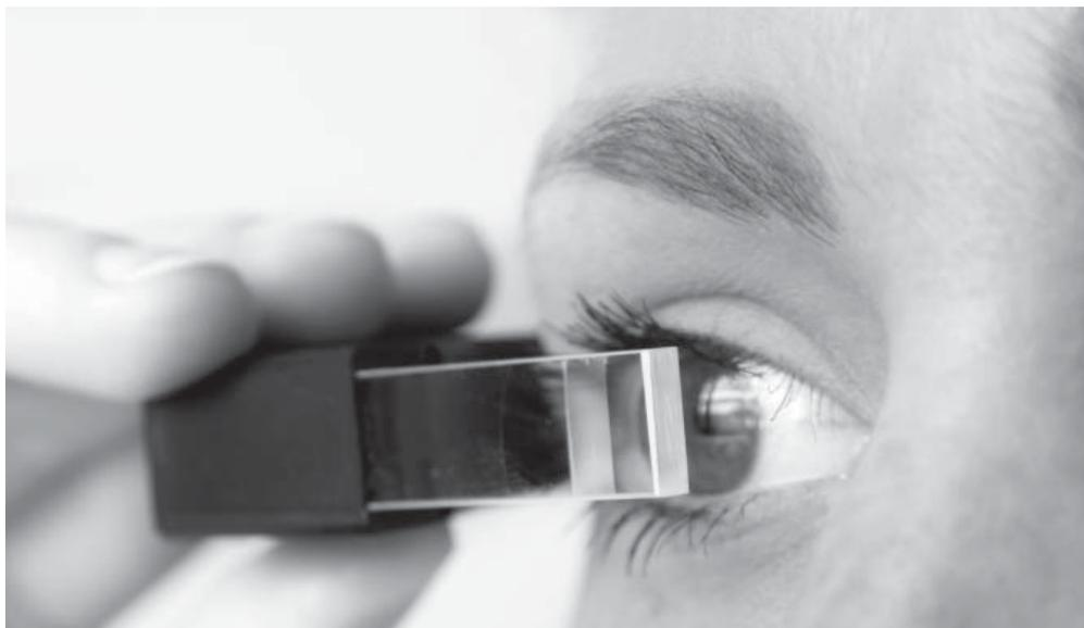
The near-to-eye display with see-through functionality facilitates a small, unobtrusive design.
