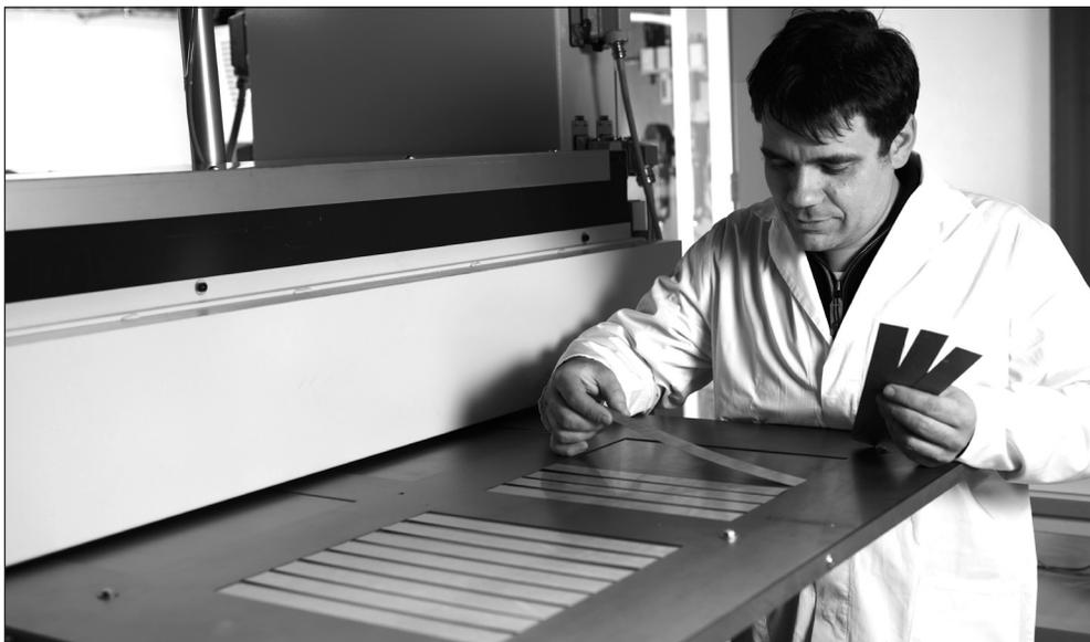
**A scientist removing samples of electrical steel from the test facility at Fraunhofer IWS; this type of material is one of the main components of transformers. (© Fraunhofer IWS) | Picture in color and printing quality: [www.fraunhofer.de/press](http://www.fraunhofer.de/press)**
