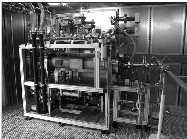
**Researchers at a new hot gas test facility are testing the waste heat use systems and turbo-chargers. Their goal is to develop more efficient powertrain concepts for passenger vehicles and trucks. (© Fraunhofer ICT) | Picture in color and printing quality: [www.fraunhofer.de/press](http://www.fraunhofer.de/press)**
