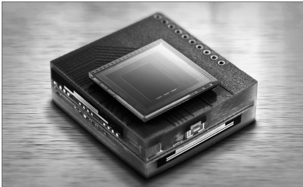
Cross-section of the microcamera module, with the image sensor mounted on the Printed Circuit board. (© Fraunhofer IZM) | Picture in color and printing quality: [www.fraunhofer.de/press](http://www.fraunhofer.de/press)
