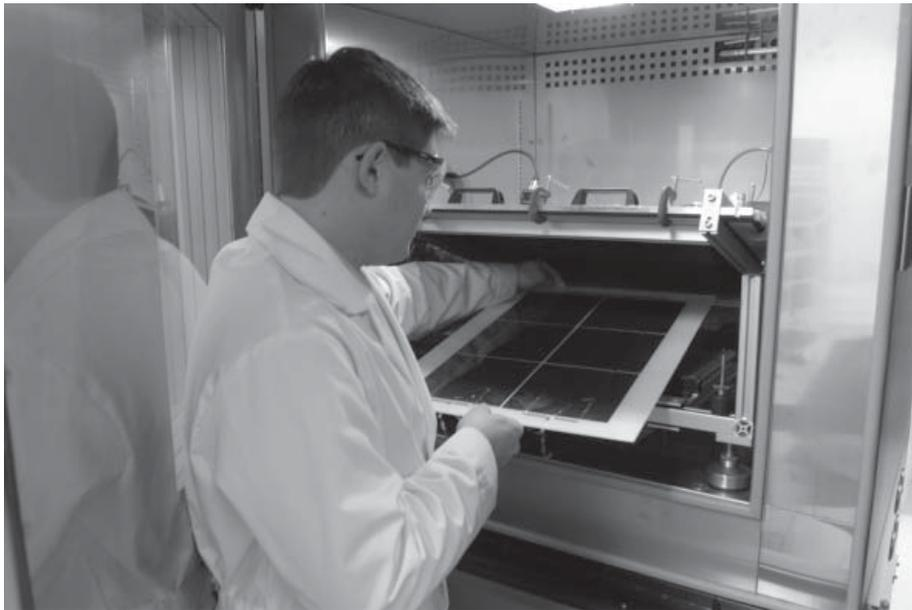
**In this mechanical test stand the researcher examines the quality of silicone-encased solar modules. (© Fraunhofer CSE) | Picture in color and printing quality: [www.fraunhofer.de/press](http://www.fraunhofer.de/press)**
