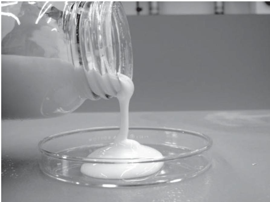
**CryoSol<sup>plus</sup>** is a dispersion that can absorb three times as much heat as water, and can prevent batteries from overheating. (© Fraunhofer UMSICHT) | Picture in color and printing quality: [www.fraunhofer.de/press](http://www.fraunhofer.de/press)
