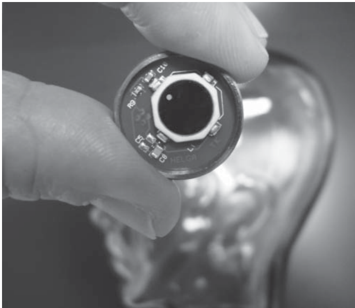
View of the not yet completely enclosed intracranial pressure sensor.
