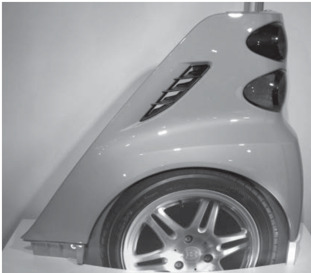
The fender with integrated LED tail light developed in the Pegasus project has been produced for demonstration purposes. (© Fraunhofer ICT)
