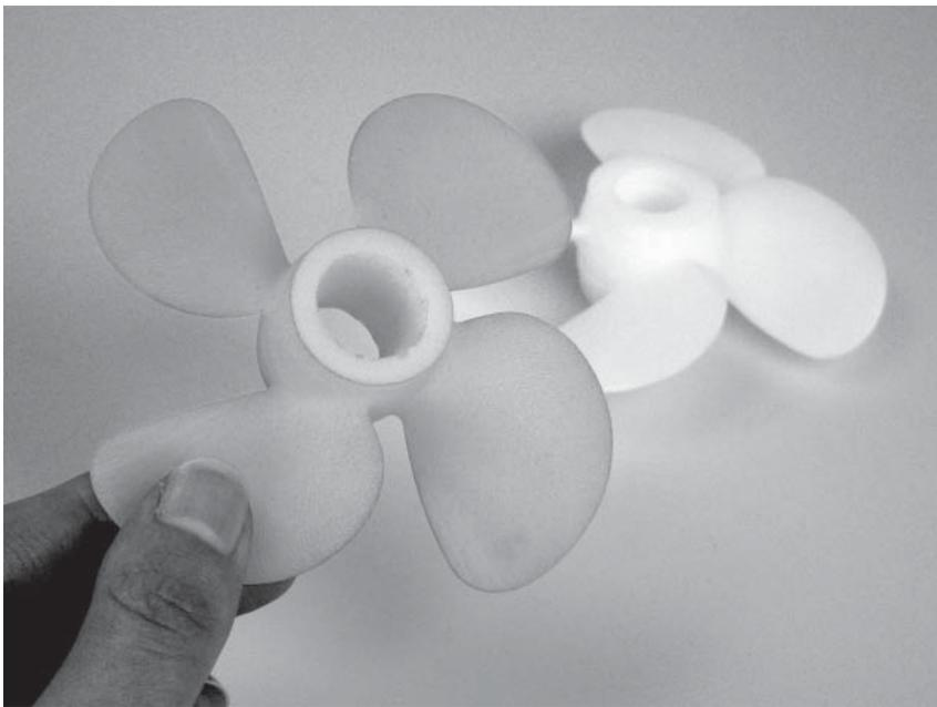
This propeller was dyed yellow in only five minutes at 90 degrees Celsius and 200 bar. At this pressure, the yellow dye powder dissolved in the CO<sub>2</sub> which transferred it into the plastic.
