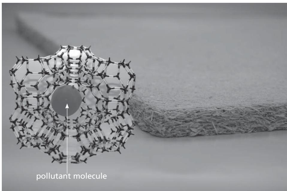
The structural model of a mineral with the dispersed pollutant molecule. When it is introduced into particleboards, the mineral reduces formaldehyde emissions from the wood material.
