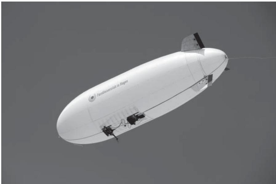
Test flight: Mounted on an airship belonging to the FernUniversität Hagen, the radiometer can detect the sources of fire even in low visibility. (© Wolfgang Krüll)
