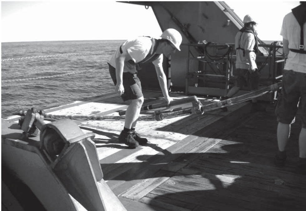
Employees put the streamer with the underwater microphones from the survey vessel into the sea. (© Fraunhofer IWES)
