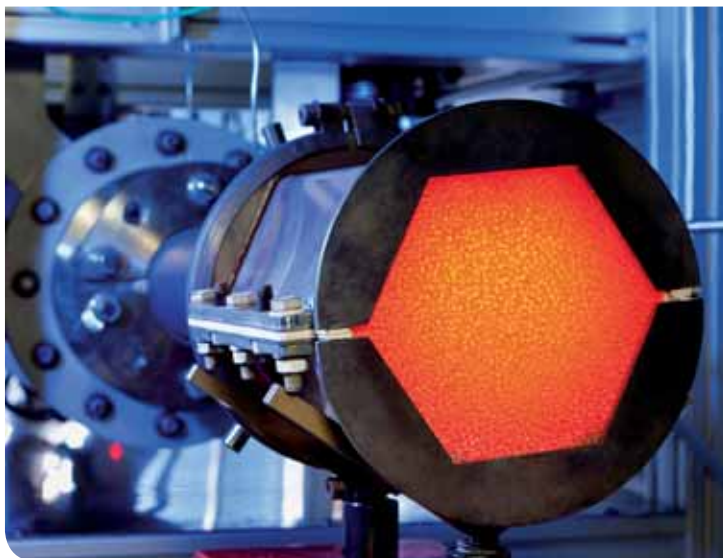
Porous ceramic filters will enable raw materials to be recovered from hot gas processes. © Fraunhofer IKTS
