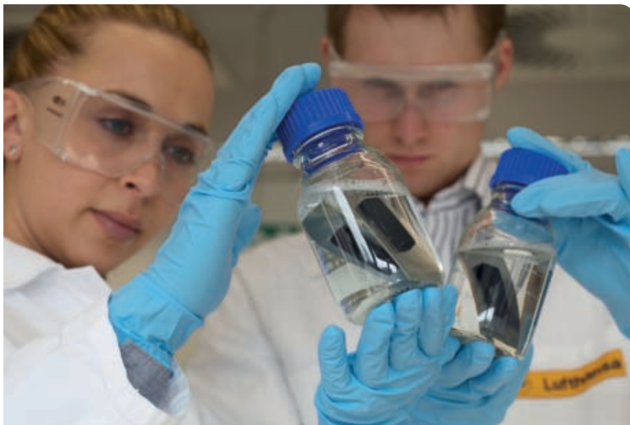
Before having its certification extended to permit its use outside the aircraft cabin, the RFID transponder had to prove its suitability in numerous tests, including for resistance to aggressive fluids. © Lufthansa Technik AG
