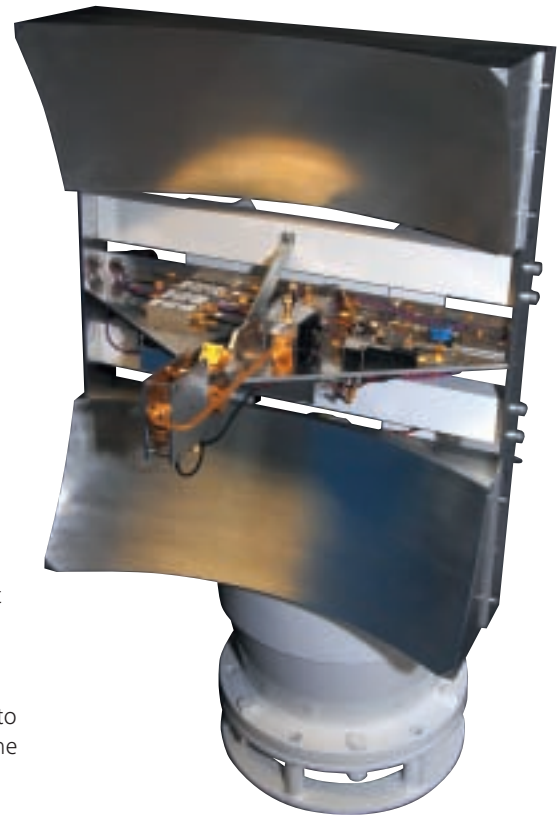
The radar sensor can detect objects that are just a few centimeters across on runways. © Fraunhofer FHR
