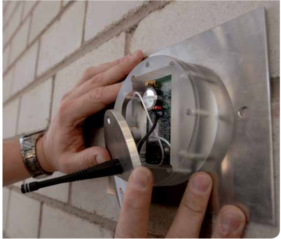
Round, wireless sensors are screwed into the wall. They record the force of the explosion.
