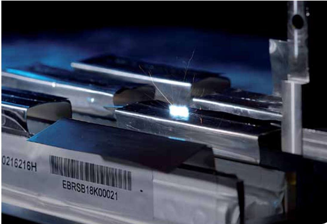
The welding of aluminum and copper battery lugs with a disk laser for the production of battery systems used in electric vehicles. © Fraunhofer ILT
