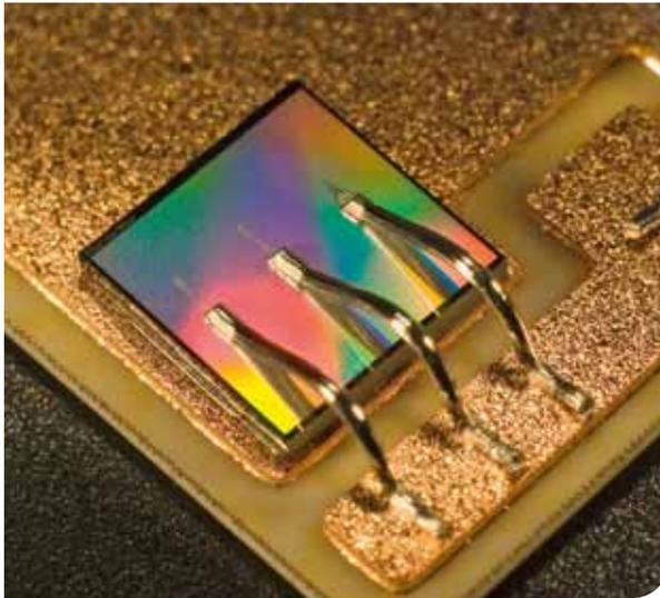
Applying electrical contacts to power semiconductors using wire bonding.
