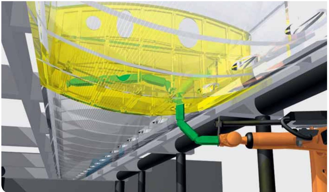
Like a snake the robot can rotate in order to reach the furthest extremities of the wingbox cavities. © Fraunhofer IWU
