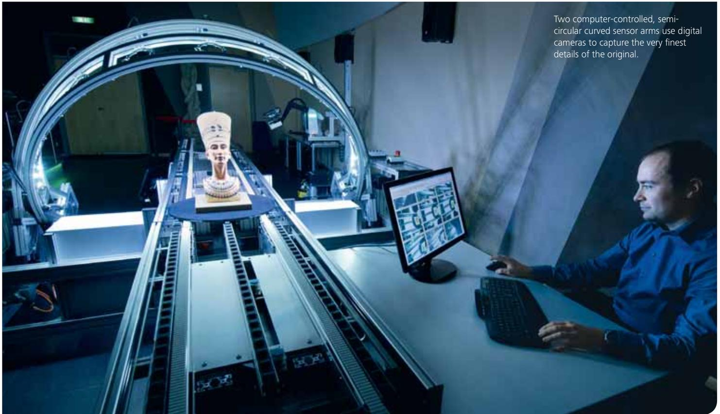
Two computer-controlled, semi-circular curved sensor arms use digital cameras to capture the very finest details of the original.
