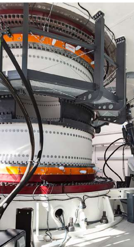
Rotor blade bearings measuring up to 6 meters in diameter are tested for offshore wind farms on the BEAT6.1 large bearing test bench at Fraunhofer IWES.
