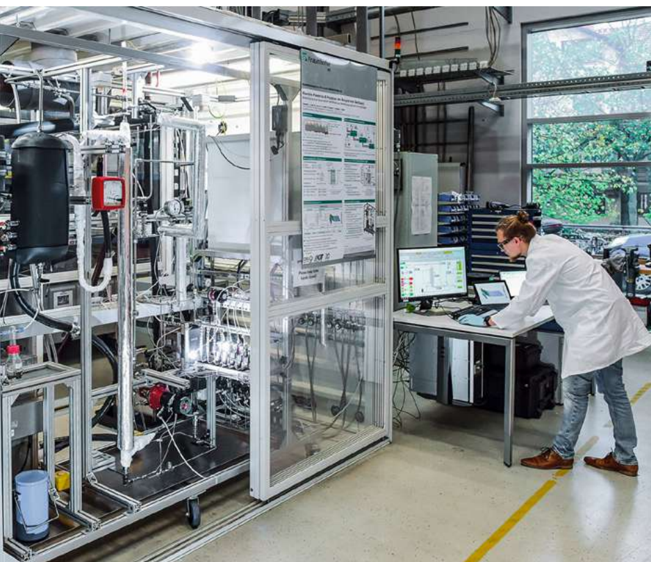
Scale-down miniplant for researching methanol synthesis at Fraunhofer ISE.
