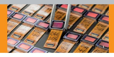
1 BIO-INSPIRED LENS ARRAY CAMERAS FOR ULTRA-COMPACT IMA-GING APPLICATIONS. Copyright Fraunhofer IOF
