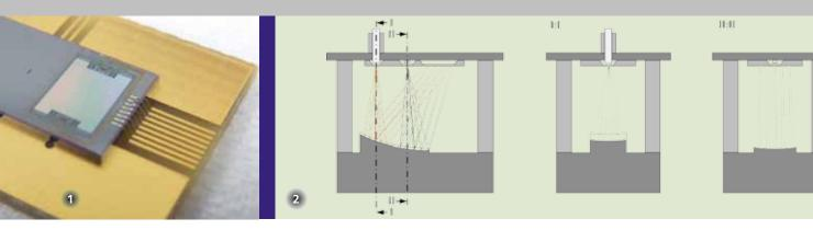
MEMS with integrated diffraction grating, driving mechanism, position detection and optical slits.
