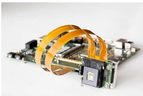
Customer Evaluation Kit with control electronics, connection cable, and 256 x 256 mirror device.
