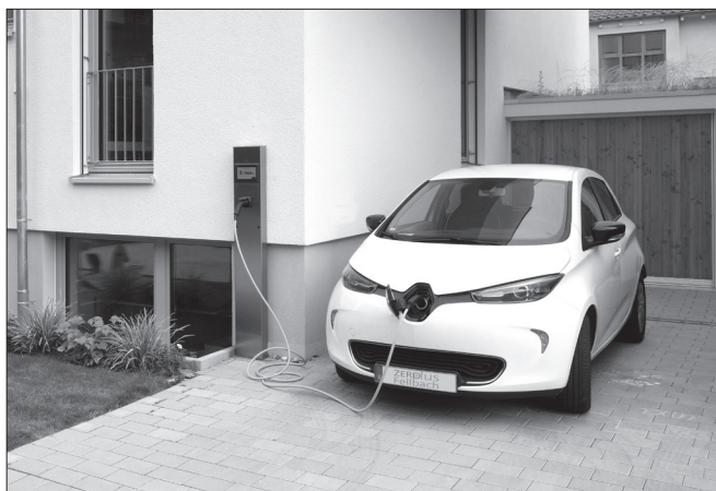
An electric vehicle is charged with photovoltaic power from the roof of the house using a charging station. (© Fraunhofer ISE) | Picture in color and printing quality: www.fraunhofer.de/press
