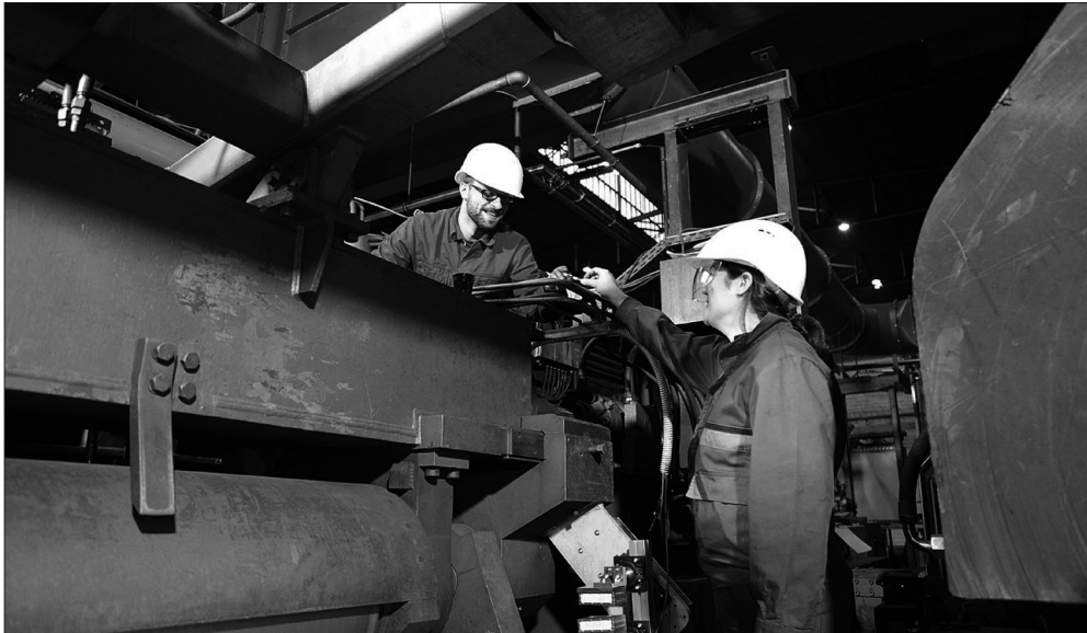
Researchers of Fraunhofer FHR installing the radar at a strip mill in Eisenhüttenstadt. (© Fraunhofer FHR) | Picture in color and printing quality: www.fraunhofer.de/press
