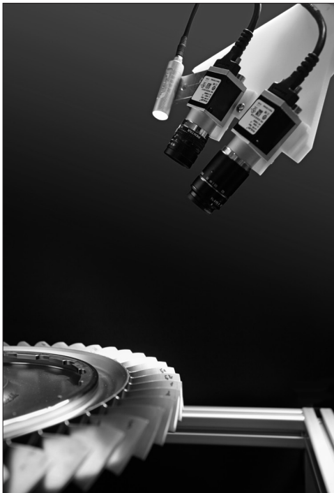
Prototypical inspection of the surface of a BLISK (Bladed Integrated Disk) with two cameras and a light source. (© Fraunhofer ITWM) | Picture in color and printing quality: www.fraunhofer.de/press
