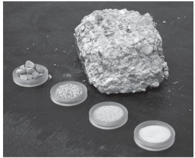
Researchers have developed a method of breaking down concrete into its constituent parts. (© Fraunhofer IBP) | Picture in color and printing quality: www.fraunhofer.de/press
