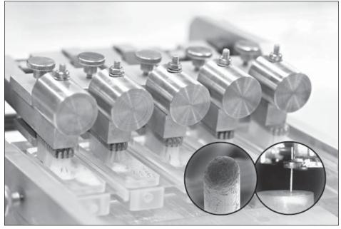
Researchers intend to supplement their microtribological analyses of the interaction between toothbrush, toothpaste and tooth surface with practical tests, using a tooth cleaning machine they have developed themselves. Bottom right: Friction and wear tests with individual bristles. (© Fraunhofer IWM) | Picture in color and printing quality: www.fraunhofer.de/press
