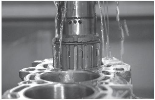
The honing tool adjusts its shape to match the piston bore holes. (© Fraunhofer IWU) | Picture in color and printing quality: www.fraunhofer.de/press
