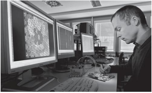
This optical wireless communication module can achieve a transmission rate of 3 Gbit/s. (© Fraunhofer IPMS/Jürgen Lösel) | Picture in color and printing quality: www.fraunhofer.de/press
