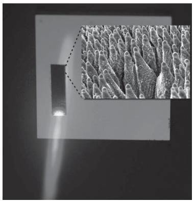
Black silicon is irradiated with a laser. Small image: Black silicon, magnified. (© Fraunhofer HHI) | Picture in color and printing quality: www.fraunhofer.de/press
