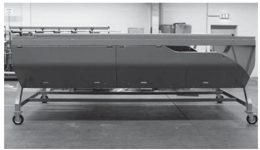
Although this diesel engine housing for trains is made of a light polyurethane-based material, it is nonetheless capable of withstanding extreme stresses. (© Fraunhofer ICT) | Picture in color and printing quality: www.fraunhofer.de/press
