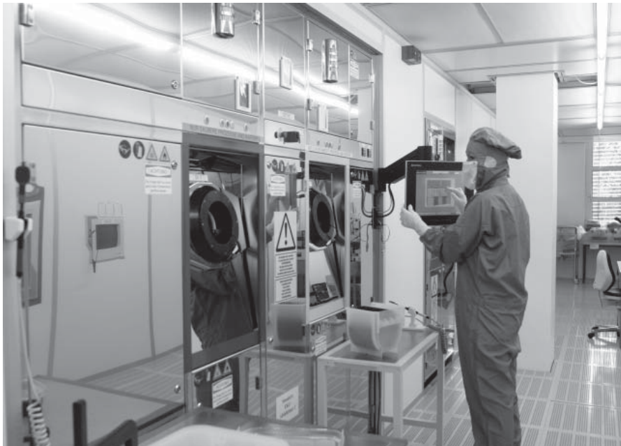
MSTs, tiny sensors integrated into semiconductor chips, are produced in the MST laboratory and clean room. A researcher operates the production machine. (© Fraunhofer IMS)
