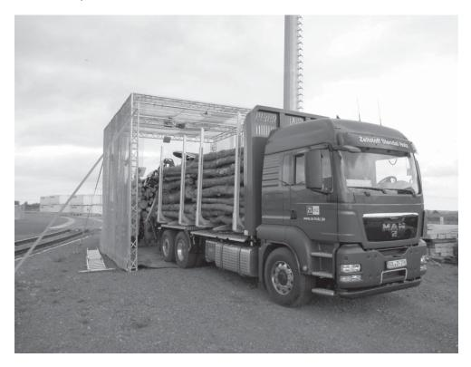
A truck passes through a special gate: Its entire truckload of timber is captured as it drives through the reader gate. (© Mike Wäsche/Fraunhofer IFF)
