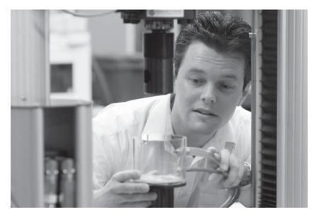
A researcher installs an environmental chamber in the special laboratory in which metals' susceptibility to stress corrosion can be tested. (© Fraunhofer IWM)
