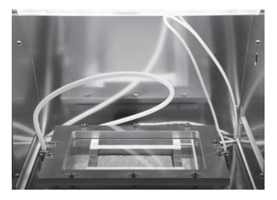
Initial tests in the measuring chamber confirm that paving slabs coated with titanium dioxide can reduce ambient nitrogen oxide levels. (© Fraunhofer IME)
