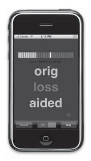
Researchers at Fraunhofer IDMT have equipped an iPod Touch with their algorithms. These can partially compensate for hearing loss among the hearing impaired. (© Fraunhofer IDMT)
