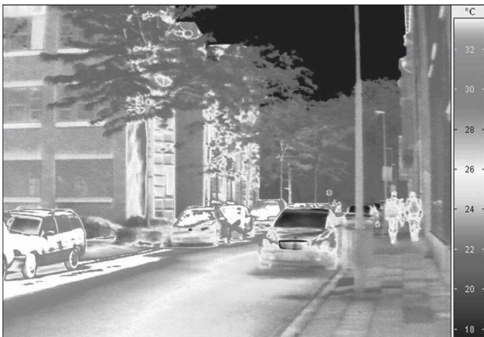
This photo was taken by an infrared camera equipped with a temperature-sensitive detector. The image shows the various temperature fields. (© Fraunhofer IMS)
