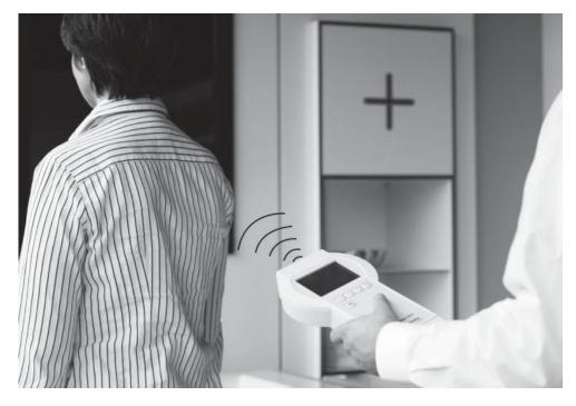
The reader device supplies the heart pressure sensor with energy. It also receives the measurement data, thereby providing doctors with information about potential cardiac malfunctions. (© Fraunhofer IMS)
