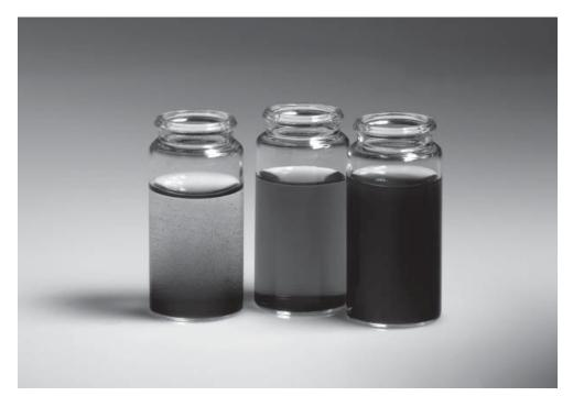
When combined with plastics, these surface-modified carbon nanotubes can, for example, improve an aircraft's protection against lightning strikes. (© Fraunhofer IFAM)
