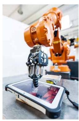
The developed robot system is capable of simulating thousands of typical usage scenarios on any kind of device with a human-machine interface, such as a touchscreen. (Source: Fraunhofer IPA/ Photo: Rainer Bez)
