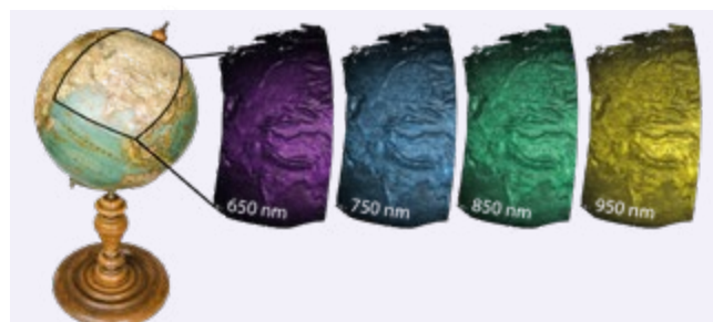
2 Multispektrale 3D-Vermessung eines historischen Reliefglobus. | Multispectral 3D measurement of a historical relief globe.
