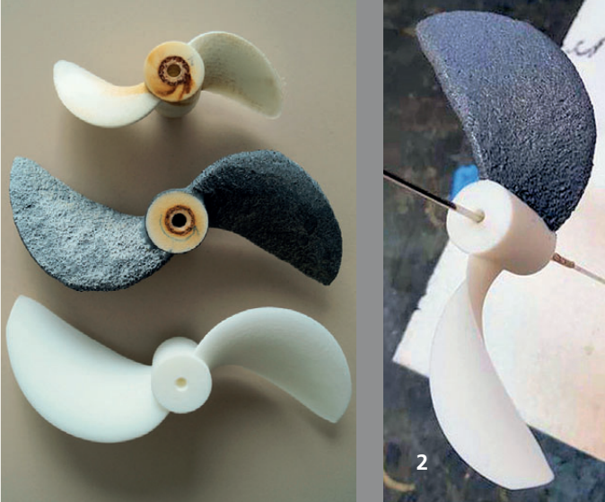
1 ● Polyamid stirrer with polymer concrete layer ■ Polyamid stirrer non-coated Test conditions: aqueous CMC suspension \varnothing_{\text{start}} = 140 \text{ mm} , n = 700 \text{ 1/min} , v_{\text{max}} = 5.5 \text{ m/s}
