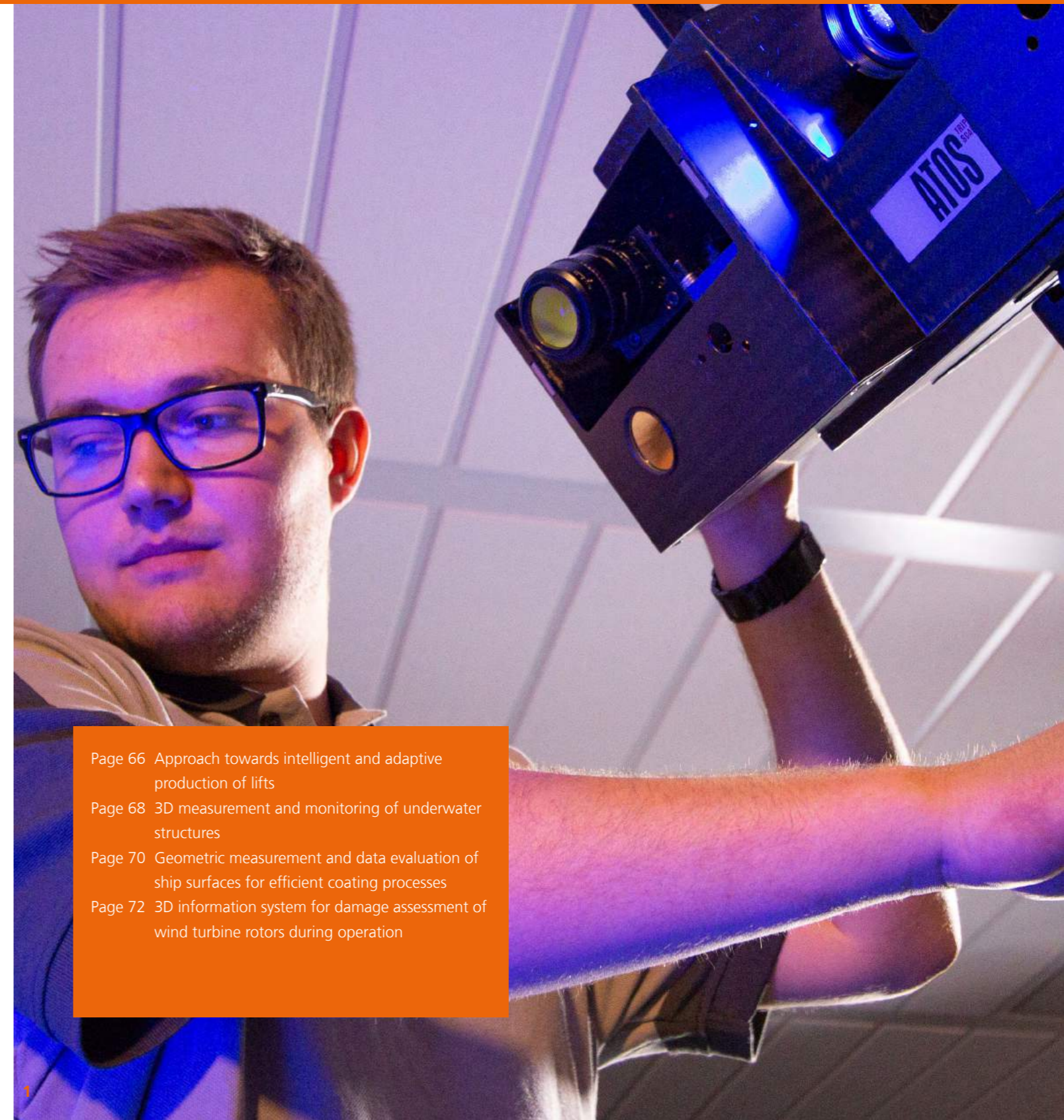
1 Lars Bretthauer during surveying with a structured light 3D scanner
