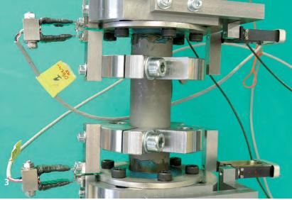
component-like samples with inhomogeneous stress states in the adhesive layer. Flange rod samples (Fig. 2) were used as component-like test samples, whereby both in-phase and phase-shifted loading could be realized.
