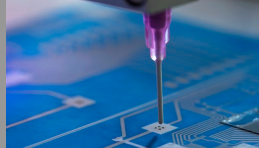
Detailed view of a foil system for temperature measurement during processing
