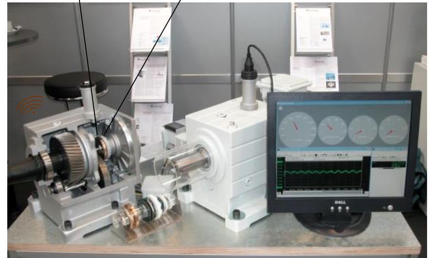
iSeal inside gear box
