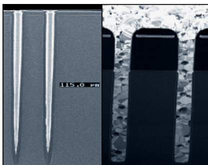
Fig. 2: TSV Copper metallization by MOCVD
